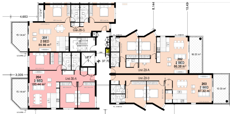
Figure 11: Typical floor plan with large balconies not only for the east facing (sea view) façade, but for units with a western aspect.
