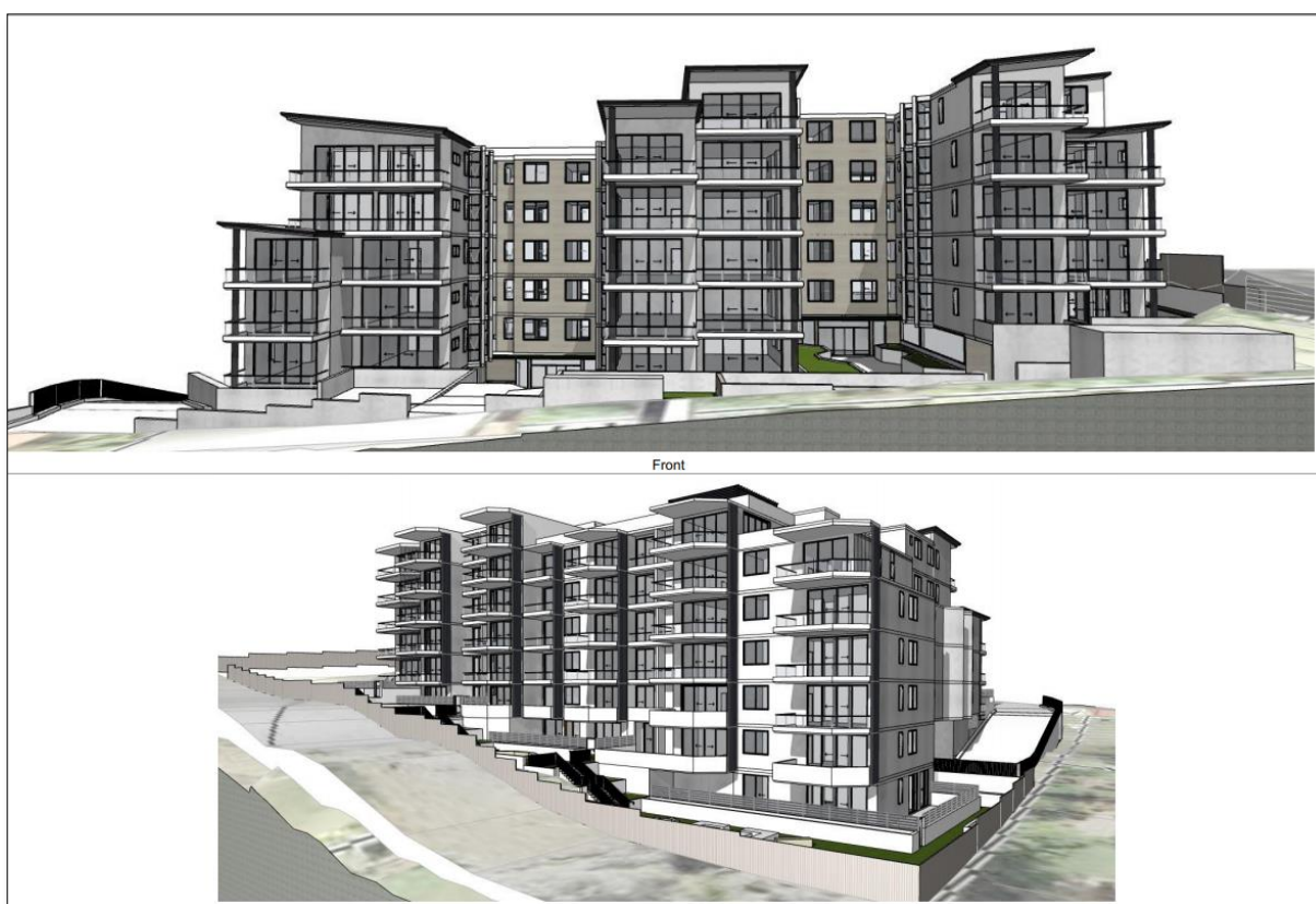
Figure 7 – Perspectives detailing building stepping with the land
